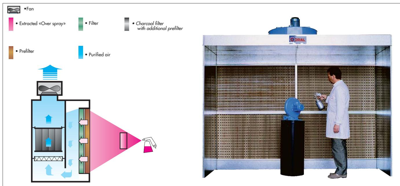
The same characteristic of the Eurodry are valid; this is the type equipped with additional charcoal filtering stage with pre-filter.
